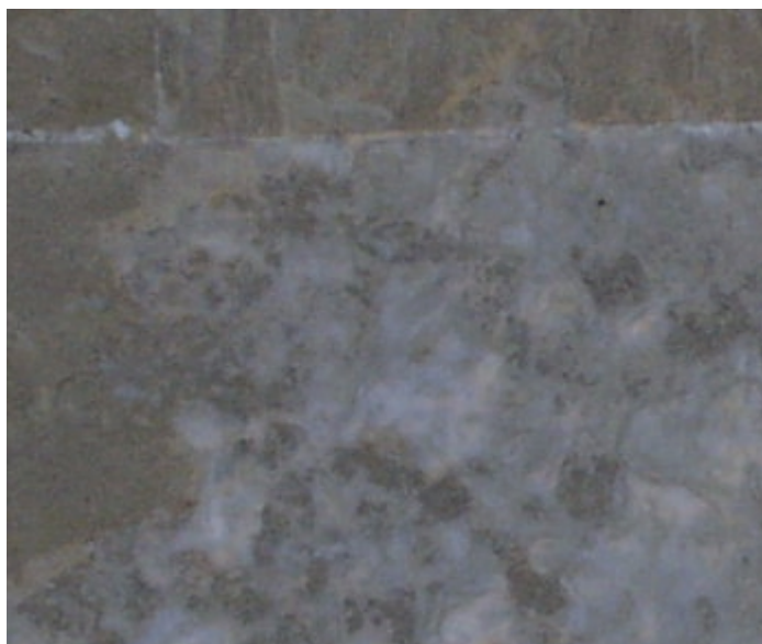
Figure 1: \text{CaCO}_3 traces on the walls of “altare dell’Annunciazione”
